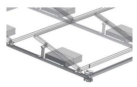
Position and connection of Front and Rear Legs, Clamps and Rail Cross Connectors.
